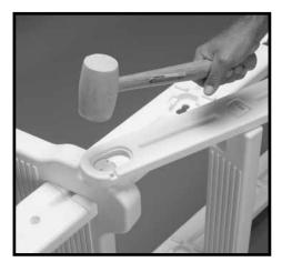
**#1:** Flex the oval openings on the Swing Ladder assembly over the two round tabs on the Platform. Using a rubber mallet tap down on the Swing-up Rail until seated over the round tab.
