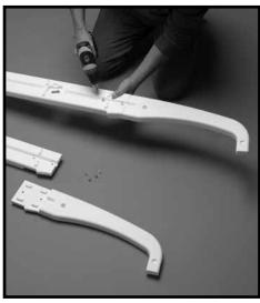
**#1:** Overlap the flat end of the Handrail onto the top of the Side Rail. Using two 1/4 - 20 x 5/8" bolts and two 1/4- 20 hex nuts, attach the Handrail to the Side Rail. Repeat for the remaining Side Rail.
