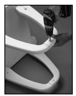
**#5:** Using two #10 x 3/4" self-tapping screws, connect the Handrails together by using one screw on the outside and one screw on the inside. Repeat for the remaining handrails.
