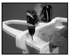
**#3:** Laying the ladder on its side, attach both Mounting Block assemblies to the ladder using two #10 x 3/4" self-tapping screws in each assembly.
